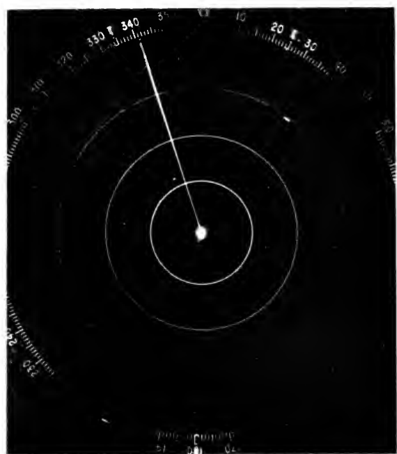
FIGURE 41.—Effect of anticlutter devices as aids to discernment of a growler from sea clutter. Top photograph shows sea return extending to 5,000 yds and a 22-foot growler at 333°T; 6,000 yards. Bottom photograph is the same situation with STC applied.
